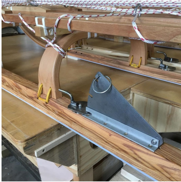
Keel plates and cow catcher fitted
