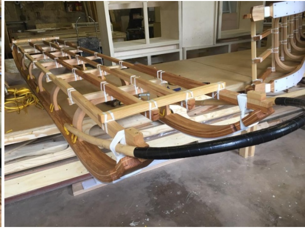
Keel plates and cow catcher fitted
